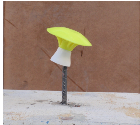
Photograph 5: Initial arrangement of the test for the second and third impact. Placement of the protective device with the maximum angle on the bar.
