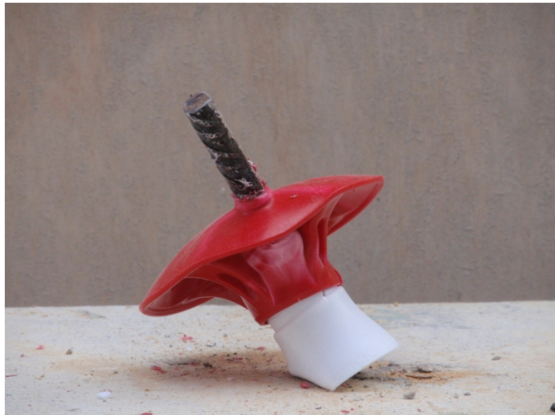
Photograph 11: State of the protective cover after performing the second impact. The protective cover was penetrated.
