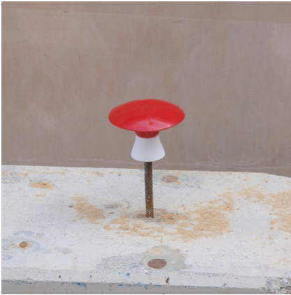
Photograph 4: Initial arrangement of the test for the first impact. Placement of the protective cover at right angles on the bar.
