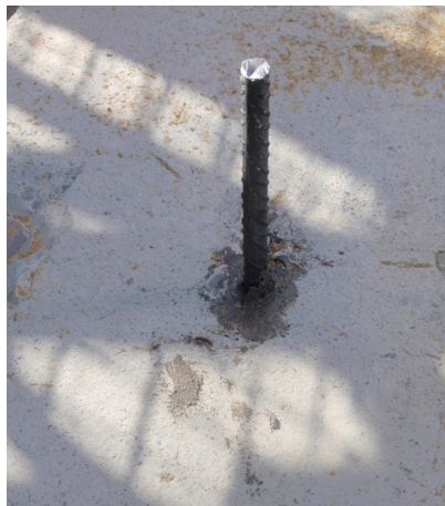
Photograph 3: Arrangement of the bar on the test supporting structure.
