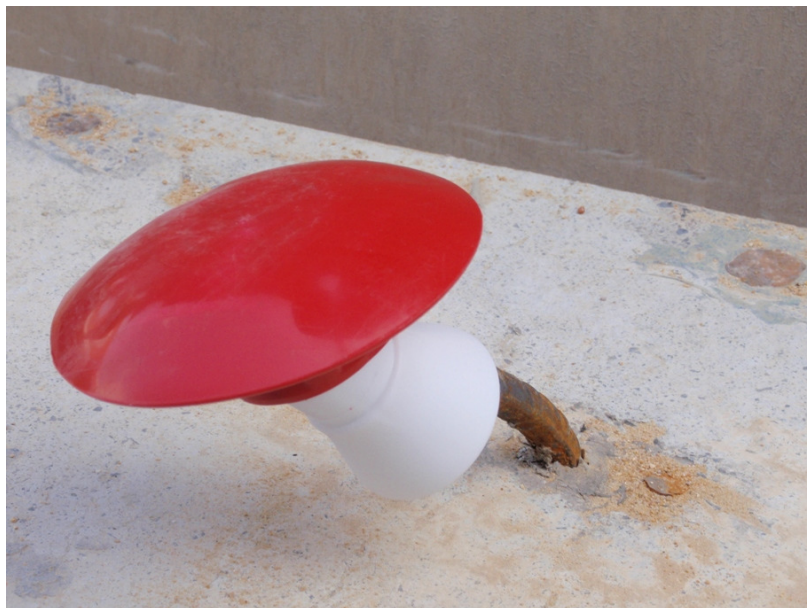
Photograph 7: Arrangement of the protective device after the first impact. No penetration of the protective cover by the bar occurred.
