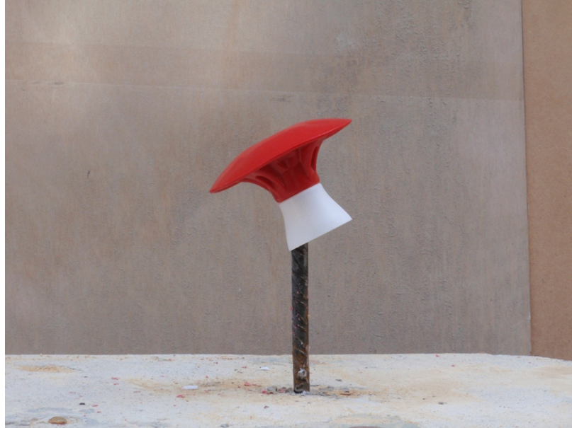
Photograph 10: Initial arrangement of the protective cover on the bar for performing the second impact.
