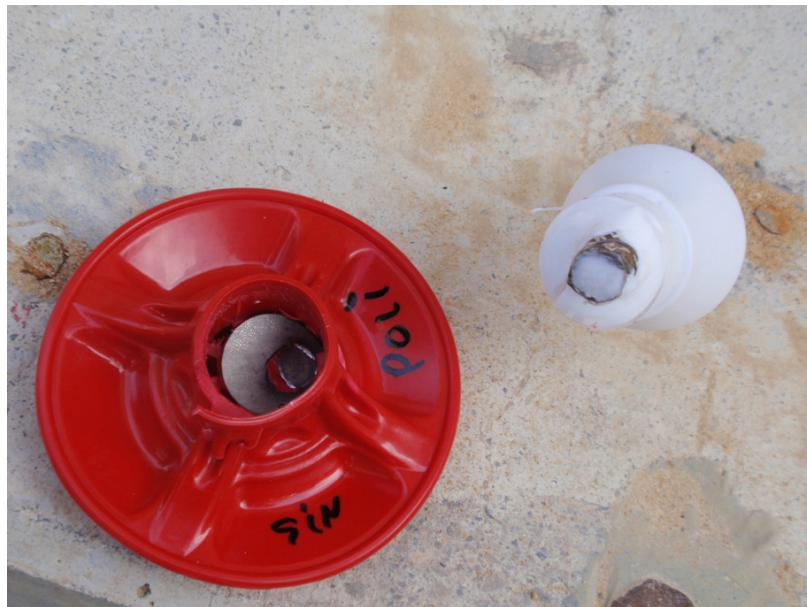
Photograph 9: Deformations and partial breaks caused inside the component.
