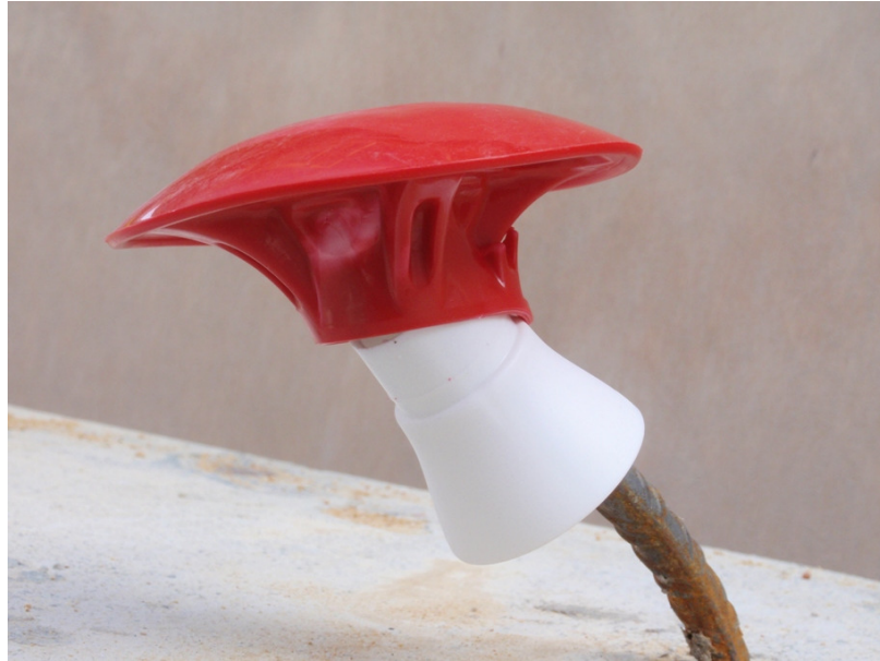
Photograph 8: Deformations and partial breaks caused in the mushroom by the impact.
