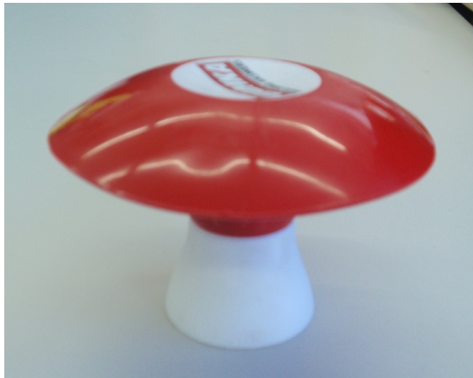
Photograph 1: Protection for reinforcement ends, object of the study.
