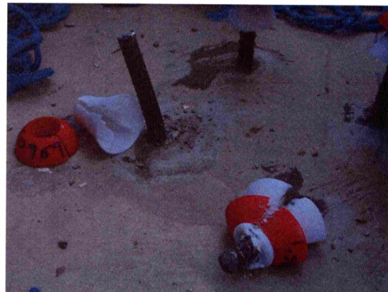
Photograph 12: Total perforation and longitudinal breakages of the protections.
