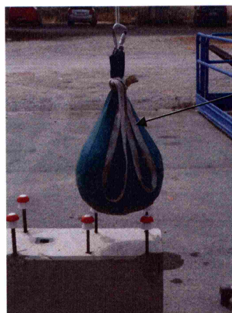
Photograph 3: Arrangement test for soft body impact.
