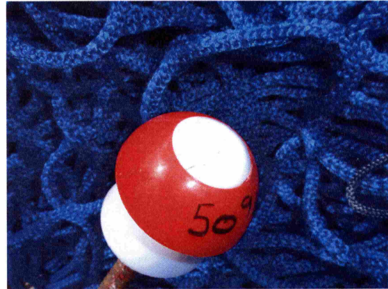
Photograph 4: Example protection in good condition after the impact.
